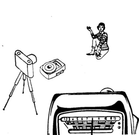
**Reflected Light Measurement:** Move the converter slide (10) all the way to the right; this uncovers the round window. The Luna-PRO is ready when the converter slide has clicked into position. Point the Luna-PRO toward the subject, as indicated by the arrow in the illustration.
