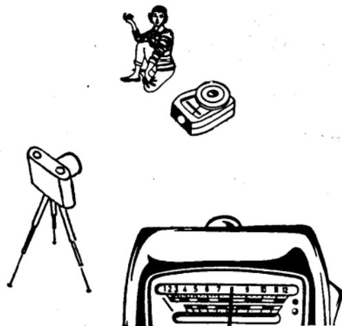
**Incident Light Measurement:** Move the converter slide (10) so that the spherical diffuser is centered over the round window. The Luna-PRO is ready when the converter slide has clicked into position. Point the Luna-PRO from the subject towards the camera, as indicated by the arrow in the illustration.
